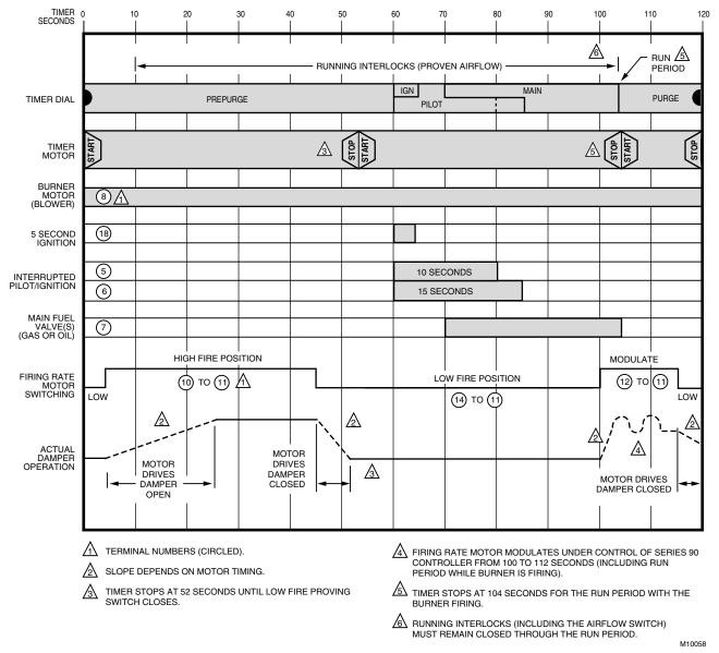
Fig. 14. Timer sequence for R4140G1148 Programmer.
